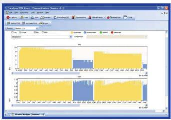
**Channel Analysis**Bits & Gain map, PSD, QLN and SNR
