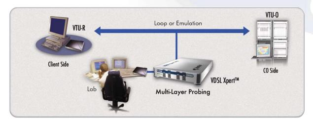
VDSL Xpert™ is easily configured at any physical location between the CO and subscriber equipment
